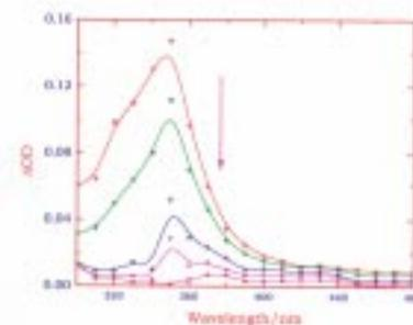
Transient absorption spectra of *p*-chloroacetophenone in acetonitrile solution at different delay times obtained using nanosecond laser flash technique. ( $\lambda_{ex} = 355 \text{ nm}$ )
