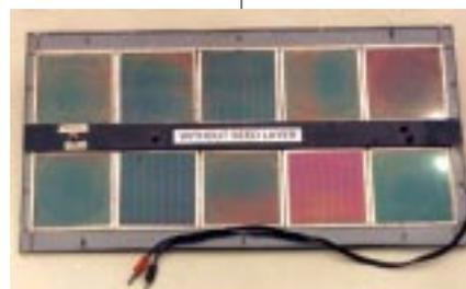
*Double junction amorphous silicon solar module
