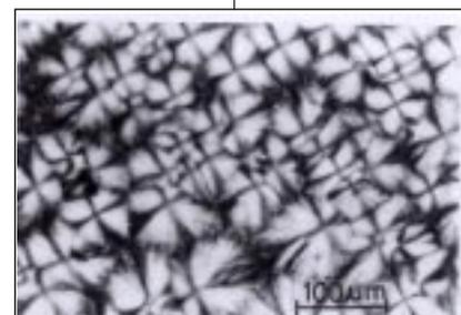
Optical micrographs of the KFE PVF<sub>2</sub> blend with PMA ( $w_{PVF_2}=0.50$ ) crystallized at 150° C for 3 days
